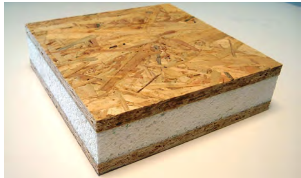
Example of a Sandwich Insulated Panel (SIP). This application would require removal and reinstallation of the exterior siding.
